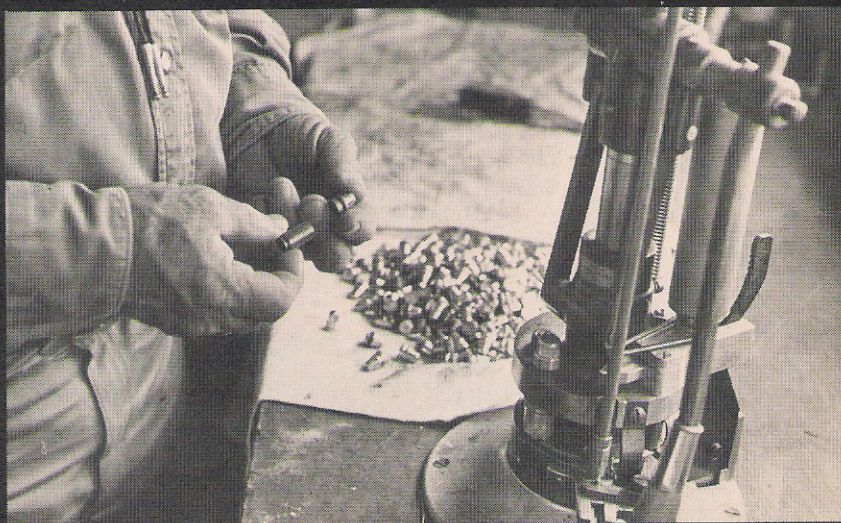
Over the years, Keith has designed cast, lubricated bullets for auto pistols as well as revolvers, such as this 200-grain hard-cast semi-wadcutter for .45 ACP. A Star press will "marry" the components after they are measured, inspected.
